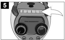
To pause playback momentarily, press the PAUSE (II) button. The tape movement stops but the tape motor is still running. Press the PAUSE (III) button again to release pause and resume recording.
