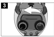
When ready to record, press the RECORD (●) button (the PLAY (►) button will automatically depress).
