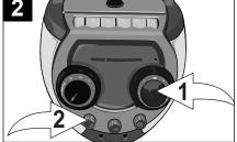
Adjust the MIC VOLUME control as desired. Increasing this control will increase the volume of the respective microphone. Adjust the ECHO control 20 to add an echo effect to your voice. The ECHO control 20 is variable so add as much or as little reverb as desired.
