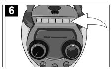
To pause playback momentarily, press the PAUSE (■) button. The tape movement stops but the tape motor is still running. Press the PAUSE (■) button again to release pause and resume normal playback.
