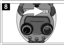
When the tape reaches the end, the auto-stop mechanism activates, the PLAY (▶) button is released and the tape motor shuts off. Press the STOP/EJECT (■▲) button to open the Cassette Door and remove the tape.
