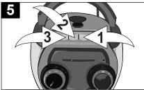
To advance or rewind the tape rapidly, press either the F.FWD (▶▶) ① or REWIND (◄◄) ② button. When you reach the desired point, press the PLAY (▶) button ③ to resume normal playback.
