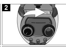
Press the STOP/EJECT (■▲) button to open the Cassette Door and insert a cassette with the open end facing the front of the unit.
