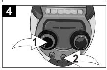
Adjust the MASTER VOLUME **1** and BALANCE **2** controls as desired. This does not affect the recording due to the ALC circuit.
