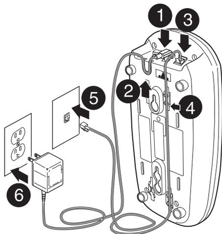
3. Plug one end of the telephone cord into the **TEL LINE** jack on the base.
