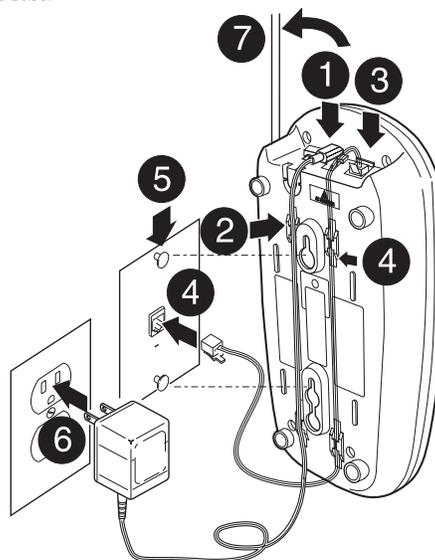
4. Place the telephone cord into the right molded channel cord holder and plug the other end of the cord into the wall jack. (*Remember, the phone must be fully charged before you can use it.*)
