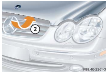
② Lever for opening the hood
