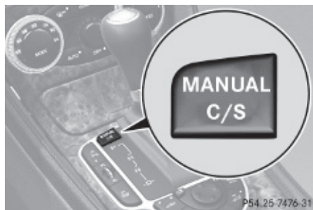
Program mode selector switch on SL 65 AMG
