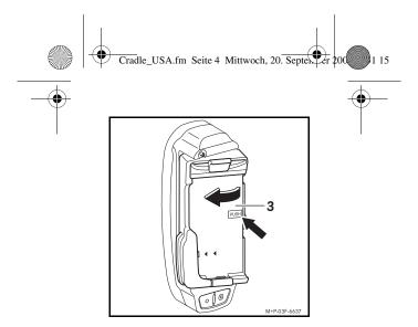
1. Push the latch (3) at the "PUSH"-sign. The latch (3) will swing out.
