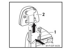
1. Insert the Mercedes-Benz V3 Cradle (1) into the latches on the pre-installed MHI contact plate (2), located in the center console.
