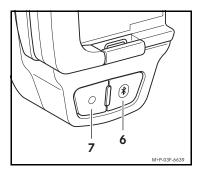
1. With Mercedes-Benz V3 Cradle connected to the vehicle press button (6) for approx. 2–3 seconds.
