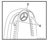
1. With Mercedes-Benz Cradle adaptor with Bluetooth<sup>®</sup> connected to the vehicle press button (3) for approx. 2-3 seconds.
