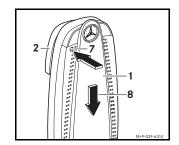
Press and hold the release button (7). Slide the Mercedes-Benz Cradle adaptor with Bluetooth<sup>®</sup> (1) in direction of arrow (8) and remove it from the pre-installed contact plate (2).
