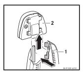
Insert the Mercedes-Benz Cradle adaptor with Bluetooth<sup>®</sup> (1) into the latches on the pre-installed contact plate (2), located in the center console. To insert the Mercedes-Benz Cradle adaptor with Bluetooth<sup>®</sup> (1), slide it upwards until it clicks into place.
