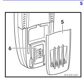
To locate the Pass-Key remove cover (5) by sliding it away from the Mercedes-Benz Cradle adaptor with Bluetooth<sup>®</sup>. Located behind this cover (5) there will be a sticker containing the Pass-Key (6).
