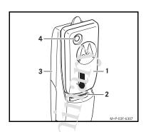
Insert the Mercedes-Jenz V60 adaptor with Bluetooth® (1) into the connector (2) to engage it into the cadle (3).
