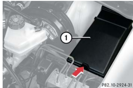
① Main fuse box
