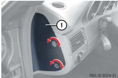
① Auxiliary fuse box
