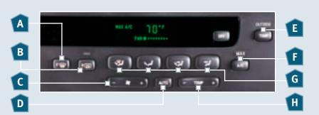
ront Window Defroster -Distributes outside air through the windshield defroster ducts. Can be used to clear ice or fog from the windshield.
