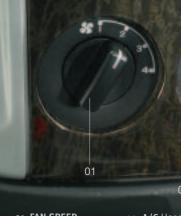
01. FAN SPEED knob to adjust the volume of air circulated in the vehicle.
