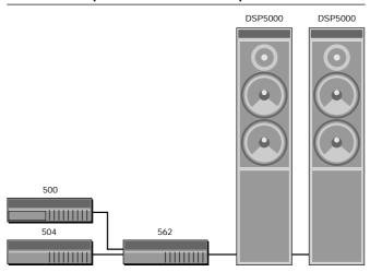
The 500 Compact Disc Transport provides a precision digital output, and can drive DSP5000 Digital Loudspeakers directly.
