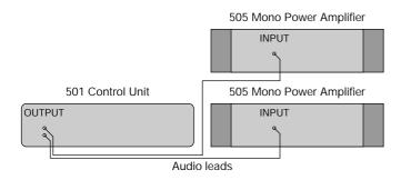
Connect the sockets marked OUTPUT L and R on the back panel of the 501 Control Unit to the INPUT socket on the back panel of each of the 505 Mono Power Amplifiers.
