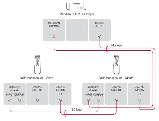
If your DSP loudspeakers do not provide Meridian SpeakerLink connections you can connect to them using the Digital and Meridian Comms connections.
