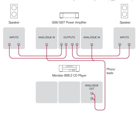
The 808.2 includes an integrated preamplifier, allowing you to connect it directly to a pair of analogue active loudspeakers, or to analogue passive loudspeakers via a power amplifier such as the G56 or G57.
