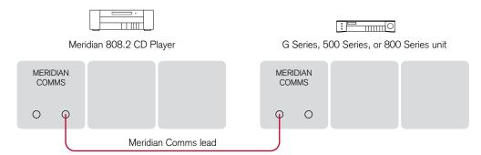
In a system of Meridian products, one of the products acts as the controller for the system, receiving infra-red commands from the MSR+ and then, if appropriate, relaying them to the other products via the Comms link.
