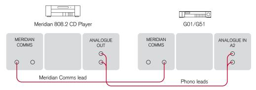
Connect the balanced or unbalanced analogue outputs to the appropriate inputs on the preamplifier.
