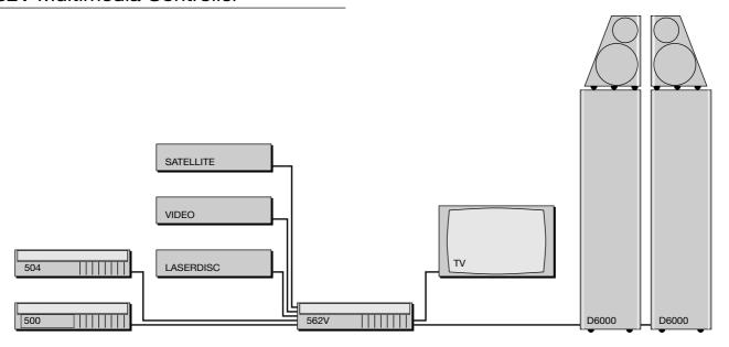
The 562V Multimedia Controller is the ideal control unit for use with the Meridian D6000 Digital Loudspeakers.
