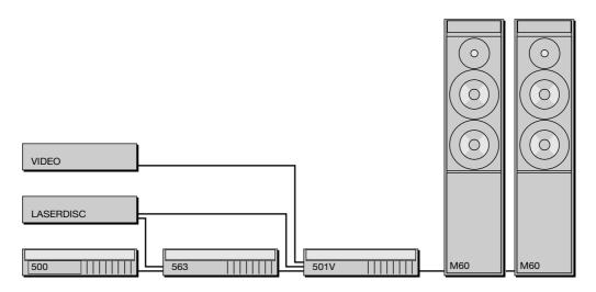
The digital output provided by the 500 Compact Disc Transport can be decoded by the 563 Digital to Analogue Converter to provide a high-quality audio output for use with a conventional audio preamplifier.
