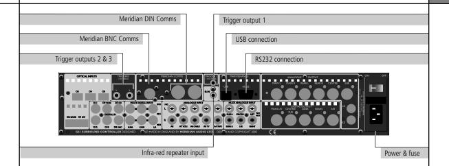
DIN COMMS Other Meridian G Series, 500 Series, or 800 Series equipment, or Meridian DSP loudspeakers.
