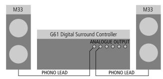
• Connect the appropriate analogue out sockets from the digital surround controller to the speaker inputs, using phono leads.
