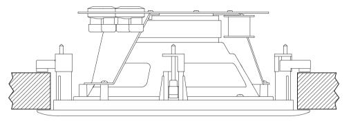
Front view of P200Z showing mounting clamps (see text):
