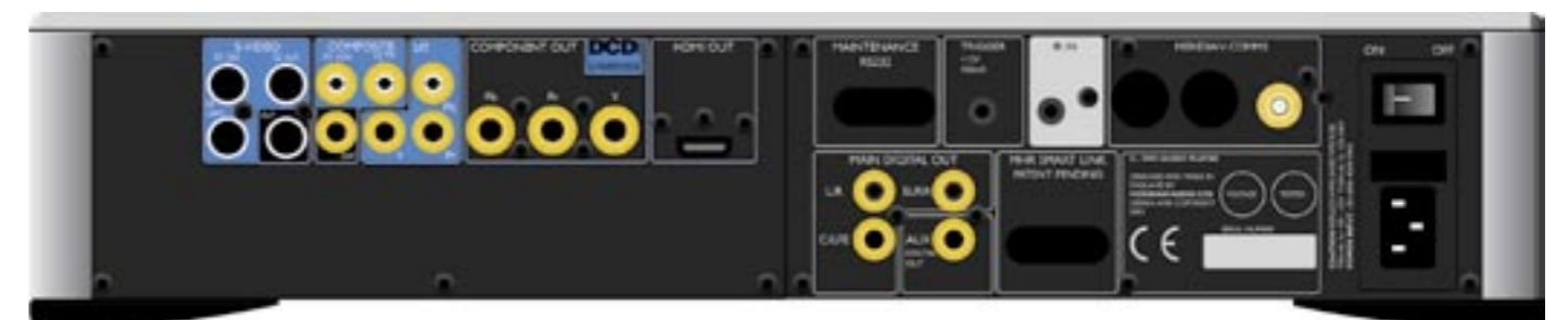
G98DH rear panel composite drawing (actual panel layout may differ slightly)
