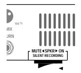
This rocker switch which is located down under the chassis and selects between the *live* "Speaker On" setting and the *silent* "Speaker Mute" setting. This is a perfect solution for *all-nighters!* This switch mutes all of the signal at the power section driver stage, removing the need for a speaker load **IN THIS POSITION ONLY!**
