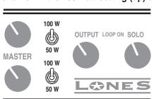
100W / 50W: Channel Power Select: channel. In the 100 watt setting (up) all four 6L6 are on line, delivering maximum power and punch. The 50 watt setting runs only the outside (far left & far right) tubes to achieve the bubbly elastic bounce only a pair of 6L6 can achieve. This powerful feature can be crucial to the sound style you wish
