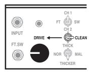
Set to CLEAN, all overdrive circuitry is removed and Channel 2 is a slightly higher gain clone of Channel 1. Because of this additional gain in what is otherwise a "rhythm" circuit, Channel 2 is an amazing solo channel for Roots style rhythm work or howling blues solo sounds. Cranking the GAIN control in Channel 2 CLEAN is a wonderful alternative to the more saturated sound of the **DRIVE** circuit.
