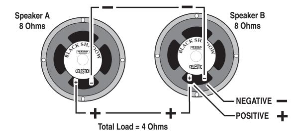
**COMBINATION OF SERIES & PARALLEL:** This is really just two sets of Series wired speakers connected in Parallel. This is how you maintain a consistent load with multiple speakers. The importance of this is more evident when you have more than one cabinet to connect to your amplifier. This is when you need to figure out the loads and how to wire them up without applying too low
