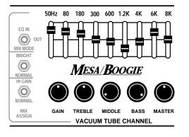
Select the VACUUM TUBE CHANNEL using the footswitch labeled TUBE on the Foot Controller and set the controls as per this example.
