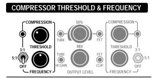
Set the Vacuum Tube Channel's Compressor Threshold and Frequency Controls per this example, while leaving the Ratio toggle switch in the  $OFF_{5:1} \bigoplus_{5:1}^{3:1}$  (down position.)
