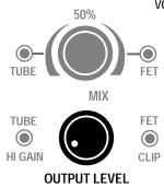
With your instrument connected to the proper Input jack (Passive or Active,) SLOWLY bring up the volume with the Output Level control while playing a note.
