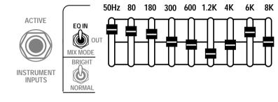
example (if you have not done so) and activate it by using — the 3 position mini toggle switch ωυτ (up position.) BK
