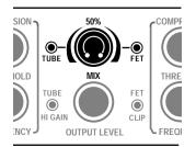
While playing a note on an open string, sweep the MIX Control from the center (Equal Blend of Tube and FET), to the left (100% Tube) and to the right (100% FET.) Between these three positions lie a myriad of unique and outrageous sounds that you will find yourself exploring for many years. The ability to combine two completely separate front end technologies allows you to "custom-build" the pre-amp of your *dreams*, by simply using the MIX Pan Pot.
