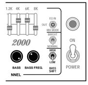
Two rotary controls, Bass and Bass Frequency enable you to center in on the region of lows that you wish to enhance and boost or cut them to your desire. Just to the right of these two controls there is a mini-toggle switch that enables you to "Shift" the region of bass that the Bass Frequency rotary control affects.
