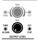
**Important...** Set the Output Level Control located in the center of the front panel to 0. (7 O'Clock)
