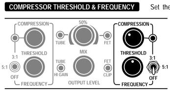
Set the Field Effect Channel Compressor's Threshold and Frequency Controls per this example, while leaving the Ratio toggle switch in the OFF  $3^{31}_{OFF}$  (down position.)
