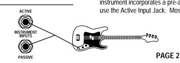
Connect your instrument to the appropriate Input jack (Active or Passive.) If your instrument incorporates a pre-amp which uses a battery for power, you will probably want to use the Active Input Jack. Most other instruments should work well with the Passive Input.
