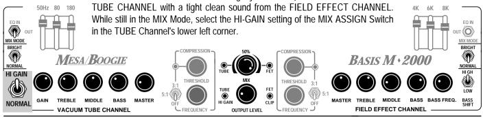
Set the controls in both channels to the setting shown in the above illustration. For this example, we have chosen a medium overdrive sound to audition. Select the MIX Mode (if you have not already done so.)
