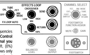
the *M-2000* 's FX LOOP MIX Control until you reach the desired blend. This scheme preserves the integrity of the attack and punch characteristics the *M-2000* is capable of delivering (when no processing is being used.) Finally, the FX LOOP AUTO ASSIGN rotary control activates the loop as well as allowing you to engage it automatically in any of the three Modes when they are called up with either the CHANNEL SELECT Rotary Control or the FOOT CONTROLLER.
