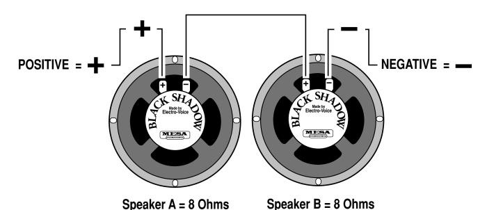
Speaker A = 8 Ohms Speaker B = 8 Ohm SERIES: Connect the Negative side of Speaker A
