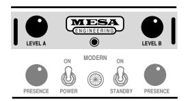
NOTE: Remember to turn the LEVEL Control to zero on any channel not connected to a speaker or load resistor! A Load must be present at all times when either channels' LEVEL Control is dialed to anything other than zero. Failure to comply to this procedure can cause serious damage to your 2:100's power section.
