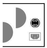
Flip the STANDBY switch to STANDBY immediately and replace the faulty power tube and the **FUSE** if necessary. If you see nothing abnormal as you lift the STANDBY switch, it is possible that a power tube shorted temporarily and blew the **FUSE**. If this is the case it may work again normally.
