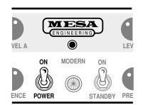
Make all necessary connections including pre-amp, effects, speakers and instrument before you flip the STANDBY switch to its ON position. AC power is turned on via the **POWER** switch and indicated by the pilot lamp. Before switching on the power, place the STANDBY switch into its Standby position and allow at least 30 seconds of warm-up time before switching the STANDBY switch to the ON position.
