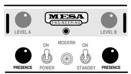
Use these **PRESENCE** Controls with discretion as they can make for some ear damaging, almost harsh sounds if set too high - especially if the TREBLE Control on your pre-amp is dialed up extremely high.
