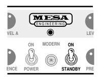
Before the power is switched on, make sure the **STANDBY** switch is in the standby position. And as mention above, wait at least 30 seconds before changing to the **ON** position.
