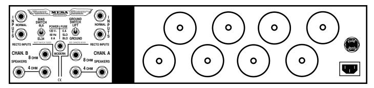
INPUTS: Located on the Rear Panel, these two 1/4" jacks are the Channel A and Channel B inputs for the 2:100. These are the inputs for pre-amps and/or effects, depending on how you have your system wired. You may drive the 2:100 with your pre-amp directly or choose to come from the last effect in a chain and drive the power amp this way. Either way is fine and up to your
