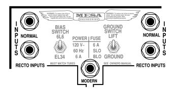
preference. The amplifier is stereo, offering two separate channels of amplification. If you wish to use only one of its channels, it is necessary to: 1) Make sure a speaker (or load resistor) remains connected to a speaker jack on both channels, including the unused one; or 2) Turn the LEVEL Control of the unused channel to zero. (This is necessary because an amplifier channel receiving any amount of signal at its input will require a "load" at its output - or damage will most likely result.)
