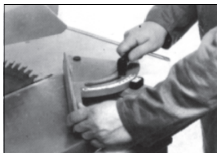
B Flip the mitre fence upwards and set for the degree required.
