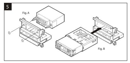
**<u>2-SHAFT HEAD UNITS:</u>** Slide the aftermarket head unit into the kit and secure with shaft nuts. (see Fig. A)
