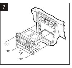
**COROLLA:** Re-connect the battery terminal and test the unit for proper operation. Mount the head unit/kit assembly to the sub-dash with (4) Phillips screws previously removed in step #1.
