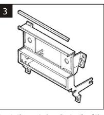
Locate the v-cut along the top lip of the Radio Housing. Using the v-cut as a guide, cut and remove the top portion of the Housing as indicated above.
