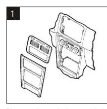
Disconnect the negative battery terminal to prevent an accidental short circuit. Unclip the radio trim bezel (upper dash). Remove (4) Phillips screws from the factory head unit, slide the unit out and disconnect the wiring. Remove the ashtray and unclip the trim bezel (lower dash). Remove (4) Phillips screws from the factory pocket/cupholder assembly and remove the assembly. (Metra recommends ordering the 88-00-8000 or 88-00-9000 to fill the space left in the upper dash location).
