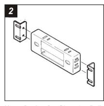
Mount Bracket Set #1 to the Radio Housing with (4) 3/8" Phillips Flat-head Screws and (4) Nuts supplied. Skip to the Installation Instructions for ALL VEHICLES on Page #7.
