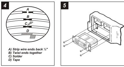
Locate the factory wiring harness in the dash. Metra recommends using the proper mating adaptor and making connections as shown. (Isolate and individually tape off the ends of any unused wires to prevent electrical short circuit). Re-connect the battery terminal and test the unit for proper operation. Mount the radio/kit assembly to the sub-dash with those screws previously removed in step #1.
