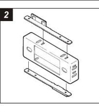
Mount Bracket Set #7 to the Radio Housing with (4) 3/8" Phillips Flat-head Screws and (4) Nuts supplied. Skip to the Installation Instructions for ALL VEHICLES on Page #7.
