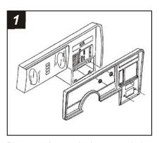
Disconnect the negative battery terminal to prevent an accidental short circuit. Remove the ashtray by disengaging the release tab at the rear of the ashtray bracket. Remove (2) screws from the lower edge of the dash trim bezel. Unsnap the top edge of the bezel and remove. Remove (4) screws securing the factory head unit and disconnect the wirina.
