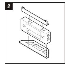
Mount **Bracket Set #2** to the **Radio Housing** with (4) 3/8" **Phillips Flat-head Screws** and (4) **Nuts** supplied. Skip to the Installation Instructions for ALL VEHICLES on Page #7.
