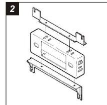
Mount Bracket Set #3 to the Radio Housing with (4) 3/8" Phillips Flat-head Screws and (4) Nuts supplied. Skip to the Installation Instructions for ALL VEHICLES on Page #7.
