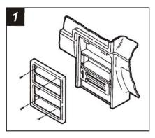
Disconnect the negative battery terminal to prevent an accidental short circuit. Open the ashtrav and remove (2) screws exposed in the ashtray cavity. Remove (2) screws from the top of the dash trim bezel. Remove the bezel. Remove (4) screws securing the factory head unit and disconnect the wiring.
