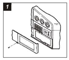
Disconnect the negative battery terminal to prevent an accidental short circuit. Remove (2) screws from the bottom of the radio trim bezel. Pry out on the edges of the bezel and remove. Remove (4) screws securing the factory head unit and disconnect the wiring.
