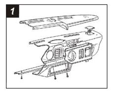
Disconnect the negative battery terminal to prevent an accidental short circuit. Open the console storage box and remove (4) screws exposed in the bottom of the box. Remove (2) screws securing the emergency brake trim and remove the trim. Unclip the gear shifter trim and remove. Open the ashtray and remove (2) screws exposed. Remove (4) screws under the ashtray opening. Remove the console. Remove (3) screws securing the factory head unit and disconnect the wiring. Contraction of the second seco
