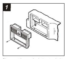
Disconnect the negative battery terminal to prevent an accidental short circuit. Remove (2) screws from the bottom of the radio trim bezel. Pry down on the (2) tabs located at the top of the radio trim bezel and remove the bezel. Remove (4) screws securing the factory head unit and disconnect the wiring.
