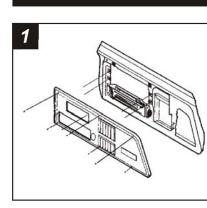
Disconnect the negative battery terminal to prevent an accidental short circuit. Remove (3) screws from the lower edge of the dash trim bezel. Remove (2) screws above the radio opening. Unsnap the right corner of the dash trim bezel, disconnect the cigarette lighter wiring and remove the bezel. Remove the screws securing the factory head unit and disconnect the wiring.
