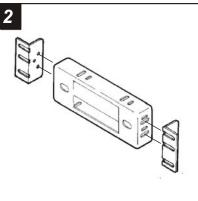
Mount **Bracket Set #4** to the **Radio Housing** with (4) 3/8" Phillips Flat-head Screws and (4) Nuts supplied. Skip to the Installation Instructions for ALL VEHICLES on Page #7.
