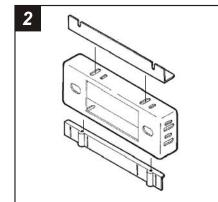
Mount **Bracket Set #5** to the **Radio Housing** with (4) 3/8" Phillips Flat-head Screws and (4) Nuts supplied. Skip to the Installation Instructions for ALL VEHICLES on Page #7.
