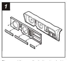
Disconnect the negative battery terminal to prevent an accidental short circuit. Remove (2) screws from the top edge of the dash trim bezel. Remove the light switch knob, cigarette lighter and ashtray. Unsnap the black trim molding under the dash trim bezel and remove (2) screws exposed. Remove the bezel. Remove (4) screws securing the factory head unit and disconnect the wiring.
