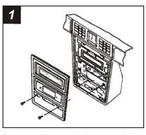
Disconnect the negative battery terminal to prevent an accidental short circuit. Remove the ashtray and climate control knobs. Remove (2) screws from the bottom of the dash trim bezel. Lift up on the bottom of the bezel and remove. Remove the screws securing the factory head unit and disconnect the wiring.
