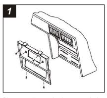
Disconnect the negative battery terminal to prevent an accidental short circuit. Remove (4) screws from the top edge of the radio trim bezel. Remove (2) screws from the bottom edge of the radio trim bezel. Remove the climate control knobs and unclip the bezel. Remove (4) screws securing the factory head unit and disconnect the wiring.
