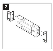
Mount Bracket Set #1 to the Radio Housing with (4) 3/8" Phillips Flat-head Screws and (4) Nuts supplied. Skip to the Installation Instructions for ALL VEHICLES on Page #7.
