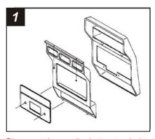
Disconnect the negative battery terminal to prevent an accidental short circuit. Remove (2) screws from the top edge of the dash trim bezel. Pull out on the top of the bezel, unhook the base and remove the bezel. If a factory head unit is NOT present, scribe the (4) mounting holes and radio opening onto the bezel. Drill the holes, cut the opening and place (4) U-clips over the mounting positions.
