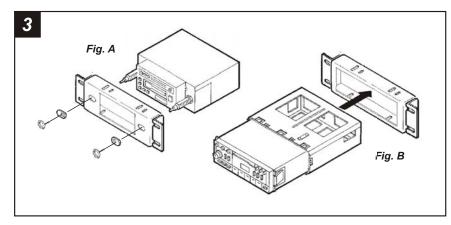
**<u>2-SHAFT HEAD UNITS:</u>** Attach the **Shaft Masks** to the **Radio Housing.** Slide the aftermarket head unit into the kit and secure with shaft nuts. (see Fig. A)
