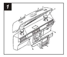
Disconnect the negative battery terminal to prevent an accidental short circuit. Open the ashtray and remove (2) screws exposed. Unclip the dash trim bezel and remove the radio dummy plate. Place (4) U-nuts over the mounting positions in the sub-dash.
