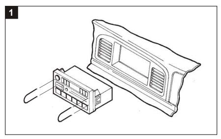
Disconnect the negative battery terminal to prevent an accidental short circuit. Using Metra's 86-5618 or AW-FDRT, pull the factory head unit from the dash and disconnect the wiring.
