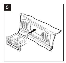
Re-connect the battery terminal and test the unit for proper operation. Mount the **Rear Support Bracket** to the back of the unit. Snap the head unit/kit assembly into the sub-dash. (Be sure the Rear Support Bracket engages the support shelf in the dash).
