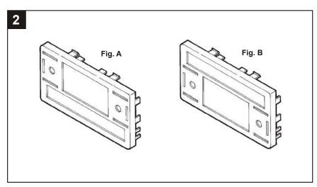
B-SERIES PICKUP, ECONOLINE, EXPLORER, MOUNTAINEER, RANGER: Position the Radio Housing with the radio opening at the TOP for the remainder of the installation. (see Fig. A)
