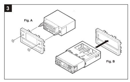
2-SHAFT HEAD UNITS: Slide the aftermarket head unit into the kit and secure with shaft nuts. (see Fig. A)
