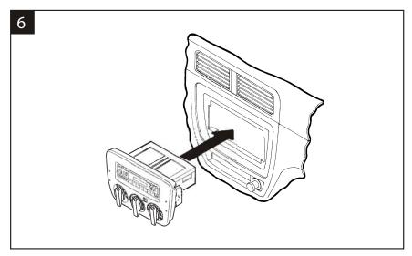
Re-connect the battery terminal and test the unit, climate controls and rear defroster for proper operation. Snap the Integrated Mounting Kit assembly into the sub-dash.
