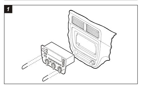
Disconnect the negative battery terminal to prevent an accidental short circuit. Using Metra's **86-5618**, pull the factory radio/climate control panel from the dash. Disconnect the audio system connectors, blower motor switch connector, vacuum hose harness, a/c damper door switch connector, and potentiometer connector. Remove the panel.
