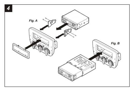
**ISO HEAD UNITS:** Snap the **ISO Faceplate** into the radio opening. Attach the **ISO Brackets** to the inner lip of the radio opening. Slide the head unit into the radio opening, align the holes in the head unit with the holes in the ISO Brackets and mount the unit to the brackets with the screws supplied with the unit. (see Fig.A).
