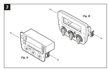
Remove (2) torx-head screws securing the mounting clips to the sides of the factory radio/climate control panel and remove the clips. (see Fig. A). Mount the clips to the **Integrated Mounting Kit** with the same torx-head screws. (see Fig. B)
