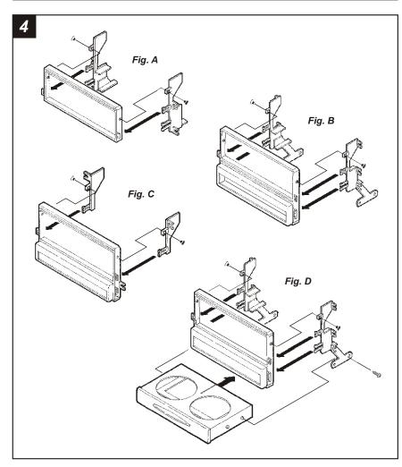
IF THE LOWER PORTION OF THE RADIO HOUSING HAS BEEN REMOVED FOR POCKET RETENTION: Mount the Brackets to the Radio Housing with (2) clips and (2) #6 x 1/4" Phillips Flat-head Screws supplied. (see Fig. A)
