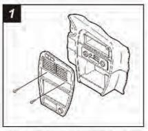
Disconnect the negative battery terminal to prevent an accidental short circuit. Remove (2) Phillips screws below the a/c vents. Pry out on the top of the dash trim bezel and remove the bezel. Remove (4) screws securing the factory head unit and disconnect the wiring.
