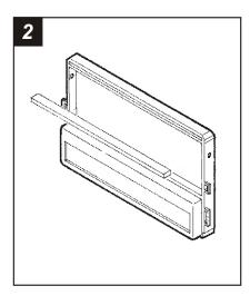
Cut and remove mounting tabs "A" and "B" on the *Radio Housing*. Cut and remove the *lower* rib from the radio opening.
