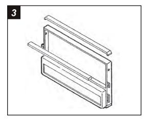
Cut and remove the lower rib from the radio opening and the top portion of the *Radio Housing*. Skip to step #5 on Page #13.
