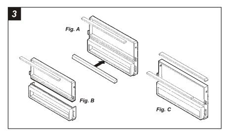
**DASH TRIM BEZELS WITH A DIVIDED RADIO OPENING:** If keeping the factory pocket is NOT desired, cut and remove the *upper* rib from the radio openingand snap the **Filler Bar** onto the bottom of the **Radio Housing.** (see Fig. A). If keeping the factory pocket is desired, cut and remove the *upper* rib from the radio opening and the bottom portion of the **Radio Housing.** (see Fig. B). Skip to the Installation Instructions for ALL VEHICLES on Page #12.
