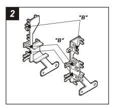
Cut and remove mounting tabs "A" and "B" on the *Radio Housing*. Cut and remove all mounting tabs on *Bracket Set #1* EXCEPT tabs "B". The mounting tabs can be identified by the stamped letter on the back of each tab.
