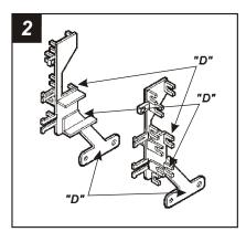
Cut and remove mounting tabs "A" and "B" on the *Radio Housing*. Cut and remove all mounting tabs on *Bracket Set #1* EXCEPT tabs "D". The mounting tabs can be identified by the stamped letter on the back of each tab.
