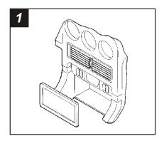
Disconnect the negative battery terminal to prevent an accidental short circuit. Using a panel removal tool, pry out on the radio trim bezel and remove. Remove (4) screws securing the factory head unit and disconnect the wiring.
