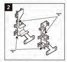
Cut and remove mounting tabs "A" and "B" on the Radio Housing. Cut and remove all mounting tabs on Bracket Set #1 EXCEPT tabs "C". The mounting tabs can be identified by the stamped letter on the back of each tab.
