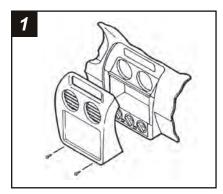
Disconnect the negative battery terminal to prevent an accidental short circuit. Remove (2) Phillips screws under the climate controls. Unclip the radio/climate control trim bezel and remove the bezel. Remove (4) Phillips screws securing the factory head unit and disconnect the wiring.
