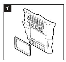
Disconnect the negative battery terminal to prevent an accidental short circuit. Unclip the radio/climate control trim bezel and remove the bezel. Remove (4) Phillips securing the factory head unit and disconnect the wiring.
