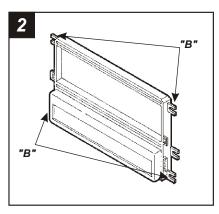
Cut and remove all mounting tabs on the *Radio Housing* EXCEPT tabs "B". The mounting tabs can be identified by the stamped letter on the back of each tab.
