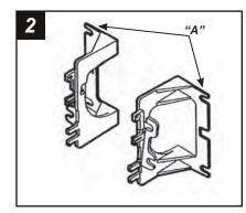
Cut and remove mounting tabs "A" and "B" on the *Radio Housing*. Locate mounting tabs "A" on *Bracket Set #3*. The mounting tabs can be identified by the stamped letter on the back of each tab.
