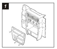
Disconnect the negative battery terminal to prevent an accidental short circuit. Remove (2) screws from the top edge of the dash trim bezel. Remove the ashtray and (2) screws exposed. Unclip the dash trim bezel and disconnect the cigarette lighter wiring. Remove (4) Phillips screws securing the factory head unit and disconnect the wiring.
