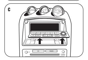
For vehicles without navigation, remove pocket mat, then remove two screws that secure switch mask. (Figure D)
