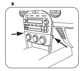
10 Pull radio/climate control panel out, disconnect plugs and remove. (Figure I)
