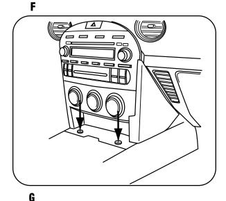
8 Carefully remove the side panels from each side of the radio/climate control panel by pulling straight back towards the rear of the car. (Figure G)
