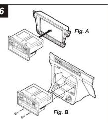
ACCORD 1990-93, INTEGRA, ODYSSEY, OASIS: Re-connect the battery terminal and test the unit for proper operation. Snap the head unit/kit assembly into the sub-dash.
