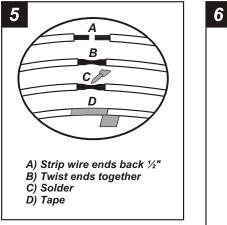
Locate the factory wiring harness in the dash. Metra recommends using the proper mating adaptor and making connections as shown. (Isolate and individually tape off the ends of any unused wires to prevent electrical short circuit).
