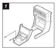
Disconnect the negative battery terminal to prevent an accidental short circuit. Remove (2) screws below the ashtray. Unclip the dash trim bezel. Disconnect the cigarette lighter wiring and remove the bezel. Remove (2) bolts securing the rear of the factory head unit and disconnect the wiring.
