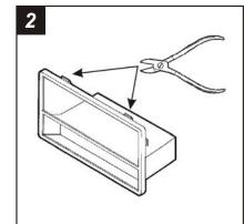
Cut and remove the *TOP* clips from the *Radio Housing.*
