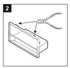
Cut and remove the *TOP* clips from the *Radio Housing.*
