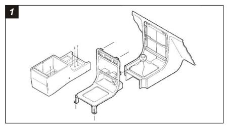
Disconnect the negative battery terminal to prevent an accidental short circuit. Remove the ashtray and (1)<sup>3</sup>/"#8 Phillips screw exposed. Open the storage compartment and remove (2) #8 Phillips screws exposed. Remove the cupholder tray and (3)#8 Phillips screws inside. Lift the center console out and remove (2) Phillips screws exposed at the base of the dash trim bezel. Unclip the bezel and remove. Remove (2) hex-head screws securing the factory head unit and disconnect the wiring.
