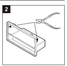
Cut and remove the *SIDE* clips from the *Radio Housing.*
