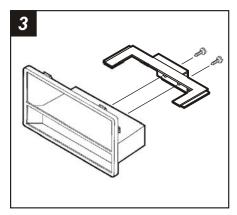
Mount the **Rear Support Bracket** to the back of the pocket with (2) **Phillips Screws** supplied. *Skip to the Installation Instructions for ALL* VEHICLES on Page #11.
