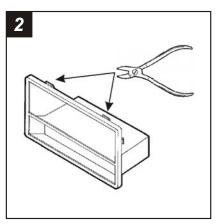
Cut and remove the *TOP* clips from the *Radio Housing.*
