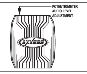
When using the CHTO-013 with a radio that has a high audio pre-out voltage, usually greater than 2 volts, the audio signal may become distorted. To resolve this follow these steps:
