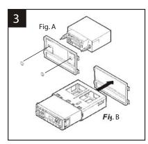
2-SHAFT HEAD UNITS: Slide the aftermarket head unit into the kit and secure with shaft nuts. (see Fig. A)
