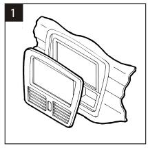
Disconnect the negative battery terminal to prevent an accidental short circuit. Unclip the dash trim bezel and remove. Remove (4) Phillips screws securing the factory head unit and disconnect the wiring.
