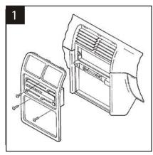
Disconnect the negative battery terminal to prevent an accidental short circuit. Remove the climate control knobs. Remove (1) Phillips screw above and (2) Phillips screws below the climate controls. Unclip the radio trim bezel. Remove (4) screws from the factory head unit. slide the unit out and disconnect the wiring.
