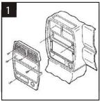
Disconnect the negative battery terminal to prevent an Remove the ashtray and (1) screw exposed. Pull out on the climate control cluster and Remove (4) screws from the VEHICLES on Page #3. factory head unit. slide the unit out and disconnect the wiring.
