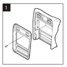
Disconnect the negative battery terminal to prevent an accidental short circuit. Remove the climate control knobs. Remove (1) Phillips screw located above the radio opening. Unclip the radio trim bezel. Remove (4) screws from the factory head unit, slide the unit out and disconnect the wiring.
