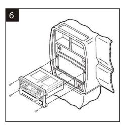
Re-connect the battery terminal and test the unit for proper operation. Slide (4) Speed Clips over the holes in the sub-dash mounting brackets and mount the head unit/kit assembly with (4) Phillips Pan-Head Screws supplied.
