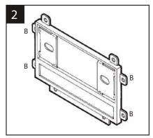
Cut and remove all mounting tabs on the Radio Housing EXCEPT tabs "B". The mounting tabs cab be identified by the stamped letter on the back of each tab. Skip to the Installation Instructions for ALL VEHICLES on Page #3.
