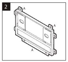
Cut and remove all mounting tabs on the Radio Housing EXCEPT tabs "A". The mounting tabs can be identified by the stamped letter on the back of each tab. Skip to the Installation Instructions for ALL VEHICLES on Page #3.
