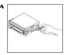
Mount the ISO Brackets to the head unit with the screws supplied with the unit. (Fig. A)
