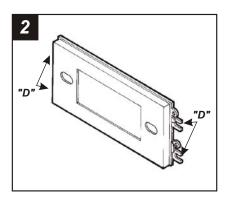
Cut and remove all mounting tabs on *Radio Housing #2* EXCEPT tabs "D". The mounting tabs can be identified by the stamped letter on the back of each tab. *Skip to the Installation Instruc-tions for ALL VEHICLES on Page #5.*
