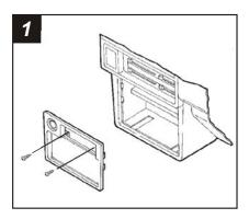
Disconnect the negative battery terminal to prevent an accidental short circuit. Remove the ashtray and (2) screws exposed in the ashtray cavity. Unclip the radio trim bezel and disconnect the wiring. Remove (4) screws securing the factory dummy plate to the back of the bezel and discard the plate.
