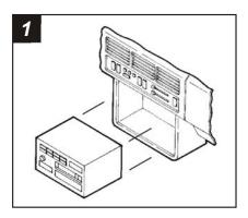
Disconnect the negative battery terminal to prevent an accidental short circuit. Reach behind the console and remove (2) nuts supporting the head unit carrier. Remove the factory head unit and disconnect the wiring..
