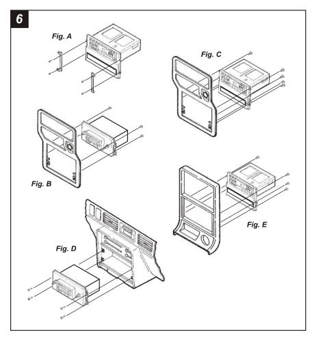
**B-SERIES PICKUP:** Re-connect the battery terminal and test the unit for proper operation. Mount Bracket Set #1 to the Housing with (4) 1/2" Hex-head Screws supplied. Mount the head unit/kit assembly to the back of the dash trim bezel with (4) screws removed in step #1 and re-attach the bezel. (see Fig. A)
