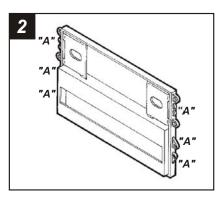
Cut and remove all mounting tabs on *Radio Housing #1* EXCEPT tabs "A". The mounting tabs can be identified by the stamped letter on the back of each tab. *Skip to the Installation Instructions for ALL VEHICLES on Page #5.*
