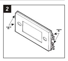
Cut and remove all mounting tabs on *Radio Housing #2* EXCEPT tabs *"E"*. The mounting tabs can be identified by the stamped letter on the back of each tab. *Skip to the Installation Instructions for ALL VEHICLES on Page #5.*
