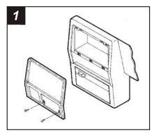
Disconnect the negative battery terminal to prevent an accidental short circuit. Remove the ashtray and (2) screws exposed in the ashtray cavity. Remove the radio trim bezel and disconnect the wiring. Remove (4) screws securing the factory head unit and disconnect the wiring.
