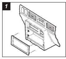
Disconnect the negative battery terminal to prevent an accidental short circuit. Gently pry out on the radio trim bezel and remove. Remove (4) screws securing the factory head unit and disconnect the wiring.
