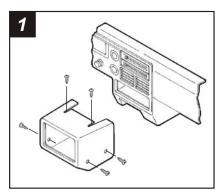
Disconnect the negative battery terminal to prevent an accidental short circuit. Remove (2) screws from each side of the radio trim bezel. Remove the ashtray and (1) screw from the rear support tab. Remove the radio trim bezel/sub-bracket assembly. Remove (4) screws securing the sub-bracket to the back of the radio trim bezel. Loosen (2) screws on top of the bezel and remove the sub-bracket from the bezel.
