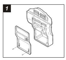
Disconnect the negative battery terminal to prevent an accidental short circuit. Remove the ashtray and (2) screws exposed. Remove the pocket and (2) screws exposed. Remove the radio trim bezel and disconnect the wiring. Remove (4) screws securing the factory dummy plate to the back of the bezel and discard the plate.
