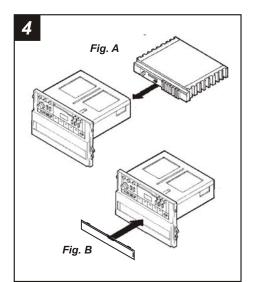
**IF AN EQUALIZER WILL BE INCLUDED:** Slide the aftermarket equalizer into the back of the **Radio Housing.** Using the hardware included with the equalizer, mount the unit to the kit. (see Fig. A)
