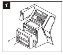
Disconnect the negative battery terminal to prevent an accidental short circuit. Remove (2) Phillips screws above the climate controls. Unclip the lower edge of the radio trim bezel and remove. Remove the screws securing the factory head unit and disconnect the wiring.
