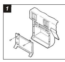
Disconnect the negative battery terminal to prevent an accidental short circuit. Remove the ashtray and the climate control knobs. Remove (3) flat-head screws from the climate control panel and remove the panel. Remove (2) Phillips screws from the top edge of the radio trim bezel. Remove (4) Phillips screws from the base of the radio trim bezel and remove the bezel. Remove (4) Phillips screws from the factory head unit and disconnect the wiring.
