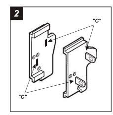
Slide *Mounting Tabs #8* into slots *"C"* on *Bracket Set #2.* The Mounting Tabs, Brackets and Bracket slots can be identified by the stamped letter on each component. *Skip to the Installation Instructions for ALL VEHICLES on Page #10.*
