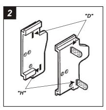
Slide *Mounting Tabs #3* into slots *"H"* and *"D"* on *Bracket Set #2.* The Mounting Tabs, Brackets and Bracket slots can be identified by the stamped letter on each component. *Skip to the Installation Instructions for ALL VEHICLES on Page #10.*
