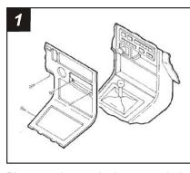
Disconnect the negative battery terminal to prevent an accidental short circuit. Remove the ashtray and (2) screws from the ashtray cavity. Remove (1) screw to the right of the steering column and (1) screw to the left of the gear shifter. Remove the screws securing the factory head unit and disconnect the wiring.
