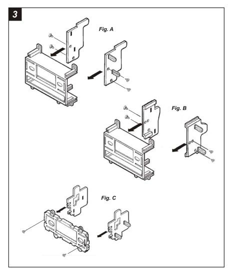
CELICA 1990-93, COROLLA (sport coupe/liftback) 1982-83, COROLLA (sedan/wagonlower dash) 1988-92, COROLLA 1984-87, LANDCRUISER 1988-92, MR2 1987-90, PICKUP 1984-88, CRESSIDA, 4RUNNER: Mount Bracket Set #1 to Radio Housing #1 with (4) Phillips Pan-head Screws supplied. (see Fig. A)
