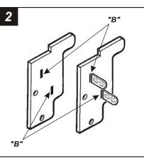
Slide *Mounting Tabs #3* into slots *"B"* on *Bracket Set #1.* The Mounting Tabs, Brackets and Bracket slots can be identified by the stamped letter on each component. *Skip to the Installation Instructions for ALL VEHICLES on Page #10.*
