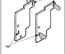
Slide *Mounting Tabs* #3 into slots "H" on *Bracket Set #1.* The Mounting Tabs, Brackets and Bracket slots can be identified by the stamped letter on each component. *Skip to the Installation Instructions for ALL VEHICLES on Page #10.*
