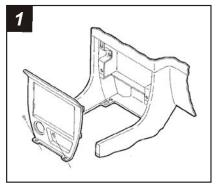
Disconnect the negative battery terminal to prevent an accidental short circuit. Pry up on the gear shifter trim panel and remove the panel. Remove (2) screws exposed on the bottom edge of the radio trim bezel. Unclip the bezel, and disconnect the ashtray and cigarette lighter wiring. Remove the screws securing the factory head unit and disconnect the wiring.
