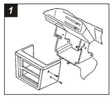
Disconnect the negative battery terminal to prevent an accidental short circuit. Remove (2) screws from each side of the dash trim bezel and remove the bezel. Remove (4) screws securing the upper radio dummy cover to the bezel and remove.
