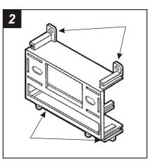
Locate the Mounting tabs on *Radio Housing #1.* (Brackets are NOT required for this vehicle). *Skip to the Installation Instructions for ALL VEHICLES on Page #10.*
