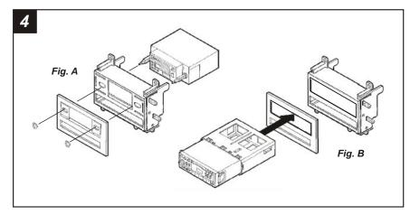
**<u>2-SHAFT HEAD UNITS:</u>** Snap the Faceplate onto the front of the Radio Housing. (For applications using **Faceplate #2**, cut and remove the bottom portion of the Faceplate). Slide the aftermarket head unit into the kit and secure with shaft nuts. (*see Fig. A*)
