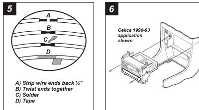
Locate the factory wiring harness in the dash. Metra recommends using the proper mating adaptor and making connections as shown. (Isolate and individually tape off the ends of any unused wires to prevent electrical short circuit).
