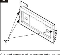
Cut and remove all mounting tabs on the **Radio Housing** EXCEPT tabs "C". The mounting tabs can be identified by the stamped letter on the back of each tab. *Skip to the Installation Instructions for ALL VEHICLES on Page #5.*
