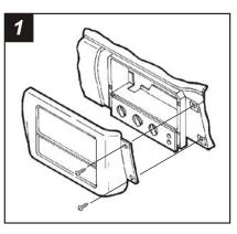
Disconnect the negative battery terminal to prevent an accidental short circuit. Open the glove box and remove (2) Phillips screws exposed on the right edge of the radio trim bezel. Unclip the bezel and remove. Remove (2) 7mm hex-head screws securing the factory head unit and disconnect the wiring.
