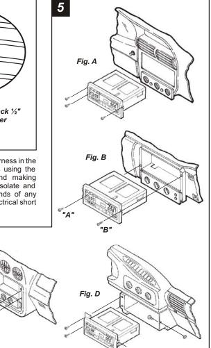
**FIREBIRD 1994-99, TRANS AM 1994-99, BONNEVILLE, GRAND AM, GRAND PRIX:** Reconnect the battery terminal and test the unit for proper operation. Mount the head unit/kit assembly to the sub-dash with (3) 7mm hex-head screws previously removed in step #1. (Run the upper-left screw through the dash plastic for the Grand Prix). (see Fig. A)
