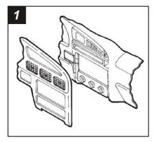
Disconnect the negative battery terminal to prevent an accidental short circuit. Unclip the entire dash trim bezel. Remove the screws securing the factory head unit and disconnect the wiring.
