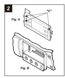
Cut and remove all mounting tabs on the **Radio Housing** EXCEPT tabs **"C"**. (see Fig. A). Using a dremel tool, cut and remove the shaded portions of the sub-dash plastic. This will provide the necessary depth for installation. (see Fig. B). Skip to the Installation Instructions for ALL VEHICLES on Page #5.
