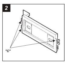
Disconnect the negative battery terminal to prevent an accidental short circuit. Unclip the radio trim bezel. Remove (4) 7mm hexhead screws securing the factory head unit and disconnect the wiring. Cut and remove all mounting tabs on the **Radio Housing** EXCEPT tabs "C". The mounting tabs can be identified by the stamped letter on the back of each tab. *Skip to the Installation Instructions for ALL VEHICLES on Page #5.*
