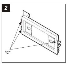
Cut and remove all mounting tabs on the *Radio Housing* EXCEPT tabs "*C*". The mounting tabs can be identified by the stamped letter on the back of each tab. *Skip to the Installation Instructions for ALL VEHICLES on Page #5.*
