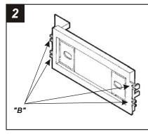
Cut and remove all mounting tabs on the **Radio Housing** EXCEPT tabs **"B"**. The mounting tabs can be identified by the stamped letter on the back of each tab. *Skip to the Installation Instructions for ALL VEHICLES on Page #5.*
