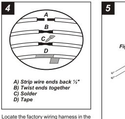
dash. Metra recommends using the proper mating adaptor and making connections as shown. (Isolate and individually tape off the ends of any unused wires to prevent electrical short circuit).
