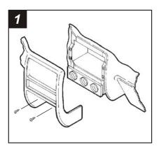
Disconnect the negative battery terminal to prevent an accidental short circuit. Remove (2) Phillips screws from the pocket. Remove (2) Phillips screws above the instrument cluster. Unclip the dash trim bezel and remove. Remove (3) 7mm hex-head screws securing the factory head unit and disconnect the wiring.
