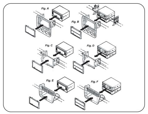
**CRV:** DOUBLE DIN HEAD UNITS: Slide the head unit into the factory bracket assembly. Align the holes in the brackets with the holes in the head unit and secure with the screws included with the unit. Cut and remove the dividing rib from the **Radio Housing** and snap the Housing into the opening (Fig. A).**Skip to step #4 on Page 11.**
