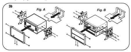
ACCORD 1994-97, CL: Secure the Mounting Bracket (mounted to the bottom of the Rear Support Tray) to the rear support provision in the sub-dash with (2) bolts previously removed. (Skip to Final Assembly on page 11.)
