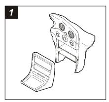
Disconnect the negative battery terminal to prevent an accidental short circuit. Remove (4) Phillips screws securing the center console. Pry out on the front edge of the console and unclip the radio trim bezel. Remove (2) Phillips screws securing the factory pocket and remove. Remove (4) Phillips screws securing the factory head unit and disconnect the wiring.
