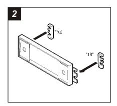
Attach Spacer 1L to the left mounting tab of the Radio Housing and Spacer 1R to the right mounting tab of the Radio Housing as shown. Skip to the Installation Instructions for ALL VEHICLES on Page #3.
