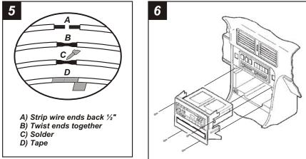
Locate the factory wiring harness in the dash. Metra recommends using the proper mating adaptor and making connections as shown. (Isolate and individually tape off the ends of any unused wires to prevent electrical short circuit).
