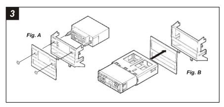
**<u>2-SHAFT HEAD UNITS</u>**: Attach the *Faceplate* to the *Radio Housing*. Slide the aftermarket head unit into the kit and secure with shaft nuts. (see Fig. A)
