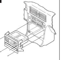
Re-connect the battery terminal and test the unit for proper operation. Mount the head unit/kit assembly to the sub-dash with (4) screws previously removed in step #1.
