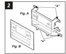
Cut and remove all mounting tabs on the **Radio Housing** EXCEPT tabs **"A"**. The mounting tabs can be identified by the stamped letter on the back of each tab. (see Fig. A). Locate **Faceplate #1**. (see Fig. B). Skip to the Installation Instructions for ALL VEHICLES on Page #2.
