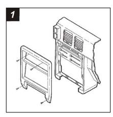
Disconnect the negative battery terminal to prevent an accidental short circuit. Remove the ashtray. Remove (2) screws from the base of the radio trim bezel. Remove (2) screws above the climate controls. Unclip the radio trim bezel and remove. Remove (4) screws securing the factory head unit and disconnect the wiring.
