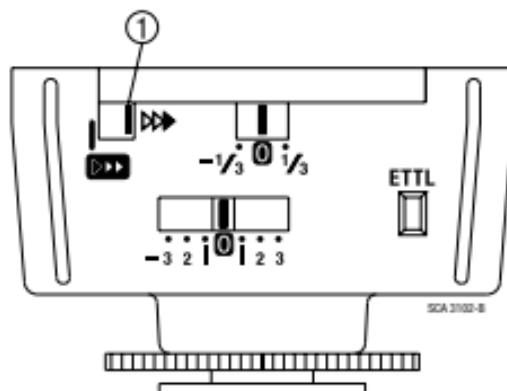
Synchronisation with the second curtain (REAR) on the SCA 3102 is always activated with the switch ① for REAR mode. This switch must be pushed into the right-hand position (see fig. below). The setting on the SCA 3102 has priority over the synchronisation mode set on the camera!
