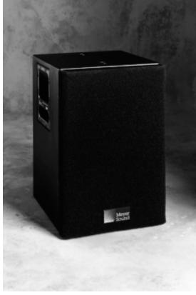
The UPL-1 and UPL-2 are two-way systems comprising a 10-inch cone low-frequency driver and 1-inch high-frequency driver housed in a vented cabinet. Both drivers are of a proprietary design, and are individually selected for maximum linearity. The high-frequency horn driver employs a titanium dome and silk suspension in a patented, low distortion design (US patent number 4,152,552). It is coupled to a 90° by 40° modified radial horn in the UPL-1, and to a 60° aspherical waveguide in the UPL-2.
