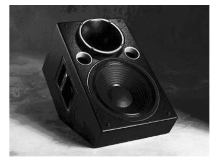
The compact speaker system shall be of the two-way type, with a 12" lowfrequency loudspeaker front-mounted in a ducted bass-reflex hardwood plywood enclosure, a compression driver mounted on a high-frequency horn which has a 1.4" throat, and a separate Control Electronics Unit.
