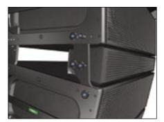
Flown and ground-stacked MILO 120 arrays and combined arrays with other M Series (MILO/M3D/M3D-Subs) models are easy to deploy using QuickFly components. Custom front and rear AlignaLinks at the cabinet corners couple the units for flying or stacking, and allow from 13 to 19 degrees of cabinet splay adjustable in two-degree increments. Because rigging connections are rigid, the array tilt is easy to adjust – often eliminating the need for a pullback strap in flown configurations.
