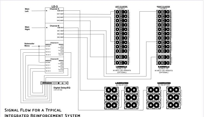
Because the MILO 120 loudspeaker is compatible with most other Meyer Sound reinforcement loudspeakers, sound designers have maximum freedom to customize systems for their needs. This block diagram illustrates the signal flow for a typical integrated sound reinforcement system using 10 MILO cabinets per side for the main arrays, and two MILO 120 loudspeakers used as downfill.
