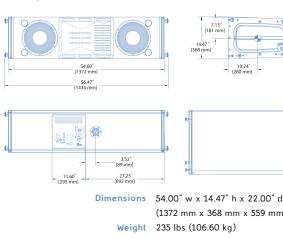
(1372 mm x 368 mm x 559 mm) Enclosure Multi-ply hardwood Finish Black textured Protective Grille Powder-coated hex-stamped steel Rigging MRF-MILO rigging frame, custom AlignaLink connectors and quick release pins
