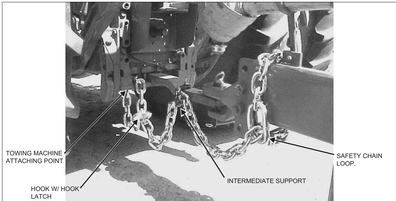
FIGURE 3. SAFETY CHAIN INSTALLATION
