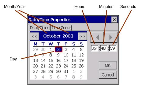
You can change the month and year using the two buttons stated (<< and >>). You can select the day directly by touching the day of the month. Hours, minutes and seconds are changed after they are selected with the buttons shown above. Hours must be entered in 24 hour format. Touching «OK» will cause the current settings in the clock module to be saved and retained, even in the event of a restart.
