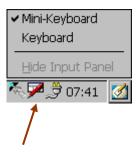
A range of different software keyboards are provided for entering characters on the device. The **«Input Panel active»** setting can be used to activate or deactivate the software keyboard. The option is deactivated by default. A change of this setting requires the system to be restarted.
