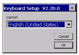
The keyboard setup – control panel makes the country setting for a USB keyboard. You can select the desired keyboard layout in the dialog shown above. The selected keyboard layout is still retained after a restart
