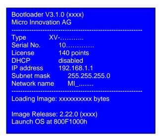
The following screen is shown first of all when the OS on the SD Flash card is started.
