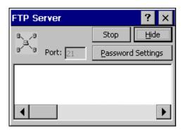
The **Hide** function is used to minimize the dialog, i.e. it is reduced to the icon inside the start bar. Double touching this icon will then cause the above dialog to be displayed again. A password protection can be activated via **Password Settings** (see <u>Password Settings</u>). Touching the **Stop** button will disconnect an active FTP connection and stop the FTP server. Touching **Start** will restart the FTP server and enables an FTP connection to be re-established.
