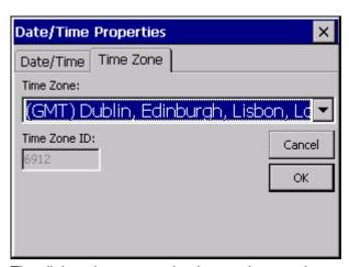
The dialog shown can also be used to set the required time zone. The «GMT» time zone is set by default, i.e. without a time shift setting. The set time zone is also retained after a restart.
