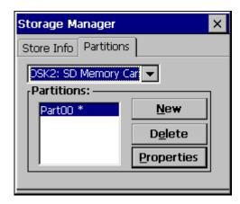
When a new partition is created, the maximum available memory space can be used, or the size can be defined in the number of sectors. MBs are converted into sectors as follows:
