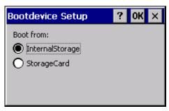
BootDevice Setup is used to specify the medium from which the panel is to start. The relevant selection options are displayed according to the features of the panel.
