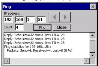
The dialog can be used to set the IP address and the number of pings. The result of the pings is output in the display field.
