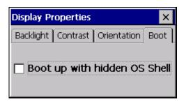
This setting can be used to modify the startup behavior of the device. If this option is enabled, either the <a href="Autoexec.bmp">Autoexec.bmp</a> bitmap or a black screen will be displayed during startup instead of the Windows CE interface. The execution of the <a href="Autoexec.bat">Autoexec.bat</a> file is also not visible.
