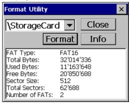
The Flash card drive can be selected in the top left selection field. The lower display field shows the information about the selected drive. This information includes details such as FAT type, total memory, currently used memory etc. Much of the information is not normally required.
