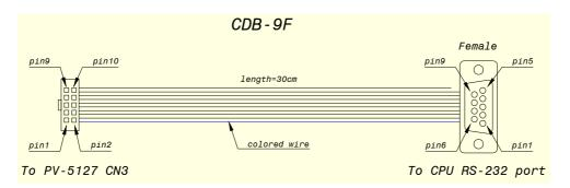
The signals use normal RS232 voltage levels. Inactive ('0') = -10V, active ('1') = +10V. In the table shown inputs are indicated by (i) and outputs by (o).
