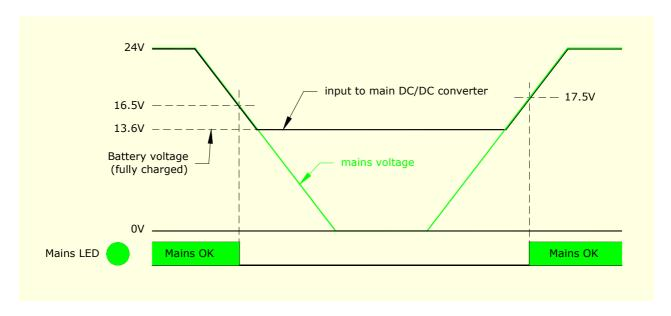
The connected lead-acid backup battery is maintained by an integrated battery charger (fast charge and trickle charge). Using an external battery temperature sensor, you can disable the charging if the battery is too hot. See the section *Battery monitor and charger*.
