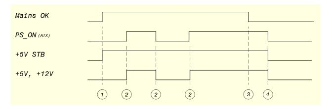
In this figure, the system temperature and the battery voltage are assumed to be OK. For the full details involving these conditions, please see the *ATX and Softoff state machines* section.
