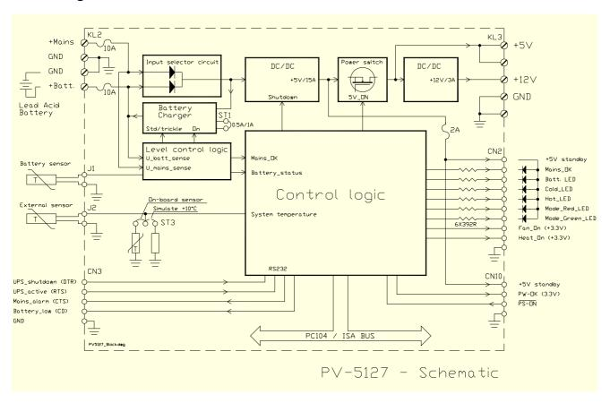
PV-5127 is built around a high efficiency DC/DC converter that converts the incoming DC voltage to 5V/15A. This output is used for +5V Standby and is available at CN2 and CN10. A power switch is used for turning on/off the output voltages +5V and +12V under software control and by the safety shutdown function.
