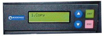
There are four buttons and an LCD on the front panel of the QD-52 duplicator.
