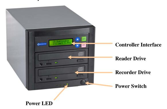
The QD-52 system consists of a CD reader, CD Writer and Controller module.
