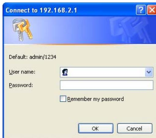
2. Please input username and password in the field respectively. Default username is 'admin' and default password is '1234', then press **<OK>** button. Once the login details are entered correctly, users can see the web management interface of this router.
