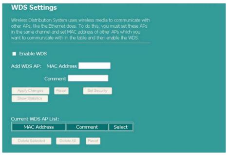
Wireless Distribution System allows the router to communicate with other APs wirelessly. To make it work, you must ensure that these APs and the Router are in the same Channel and add these APs MAC Address and Comment values into the WDS list. Don't forget to enable the WDS by clicking the check box of "Enable WDS" and pressing "Apply Changes" button to save.
