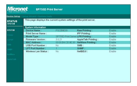
System Information includes "Device Name", "Print Server Name", "Model Type", "Firmware Version", "MAC Address" and the protocols enabled status, etc.
