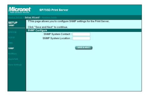
The print server supports SNMP configuration. If it is enabled, please set up the following parameters.
