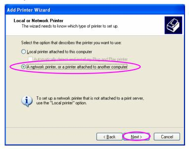
Step5. Select "Connect to a printer on the Internet or on a home or office network" and enter the URL of print server. The URL format is "http://IP:631/Port Name". The IP should be the print server's IP. The number 631 is IPP standard port number. Port Name is the port name of print server that your printer is connected to. The default port name is "Ipt1". One example of the URL is http://192.168.3.66:631/lpt1. After entering the URL of print server, click "Next".
