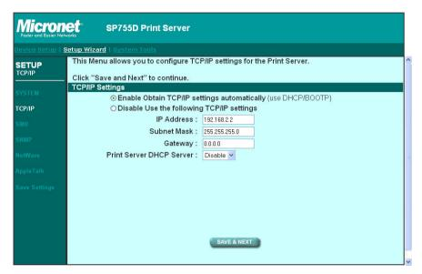
You can configure the print server to automatically get IP from DHCP server or manually specify static IP. The print server also has a built-in DHCP server. You can enable this DHCP server and let it manages IP for you.
