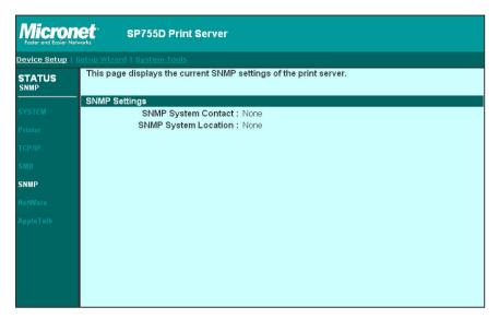
This page lists the SNMP settings of the print server. It includes the settings of "SNMP System Contact" and "SNMP System Location".
